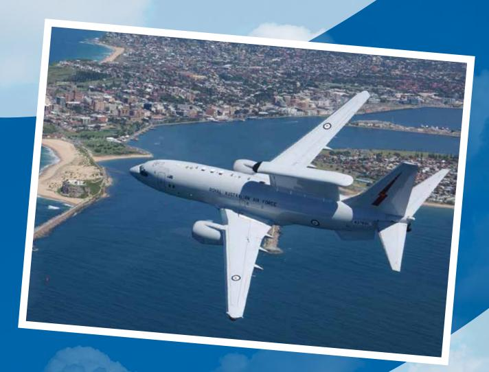
This airborne early warning and control aircraft was developed for the Royal Australian Air Force using the 737 airframe, and is also being acquired by South Korea and Turkey. Unlike the aging E-3 AWACS planes in the U.S. fleet, which mechanically rotate their radars to achieve 360-degree coverage, the lighter Australian aircraft employs a fixed radar that is electronically scanned.
