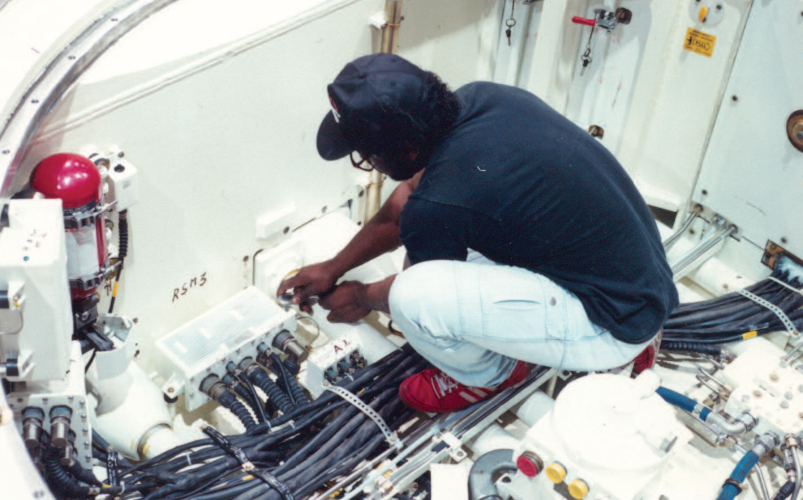
Electrical work on armored vehicle, Anniston Army Depot.
