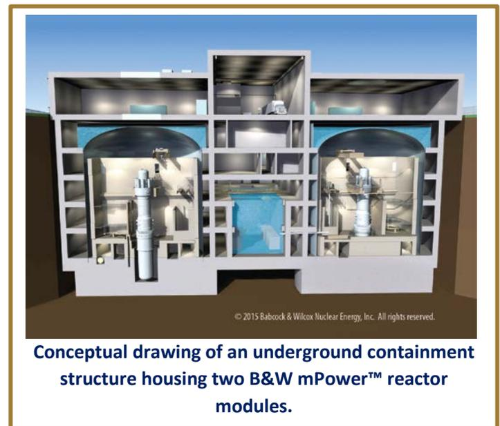
**Conceptual drawing of an underground containment structure housing two B&W mPower™ reactor modules.**
