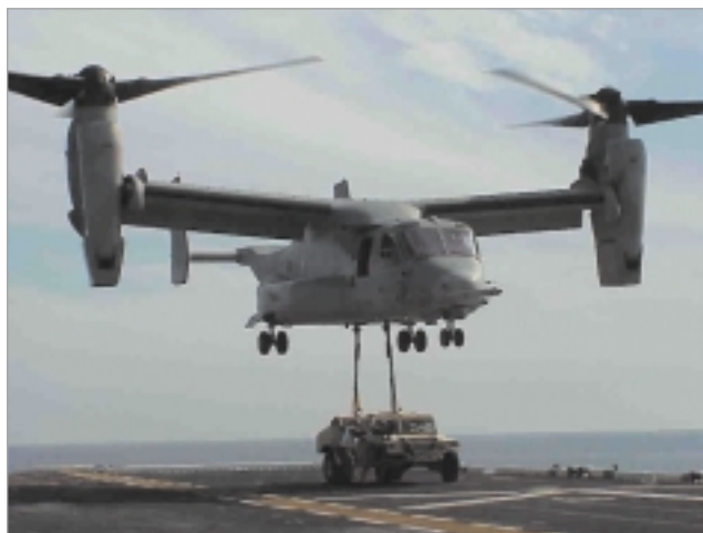
The V-22 Osprey can lift artillery and vehicles over considerable distances, such as the Humvee pictured above.
