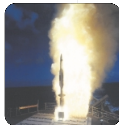
The Navy is testing a higher-speed variant of the Standard missile, the SM-3 with a third stage motor and the lightweight exo-atmospheric projectile (LEAP), a hit-to-kill warhead.
